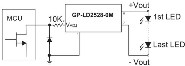
The diode and resistor suppress possible high amplitude negative spikes on the ADJ input resulting from the drain-source capacitance of the FET. Negative spikes at the input to the device should be avoided as they may cause errors in output current, or erratic device operation.
