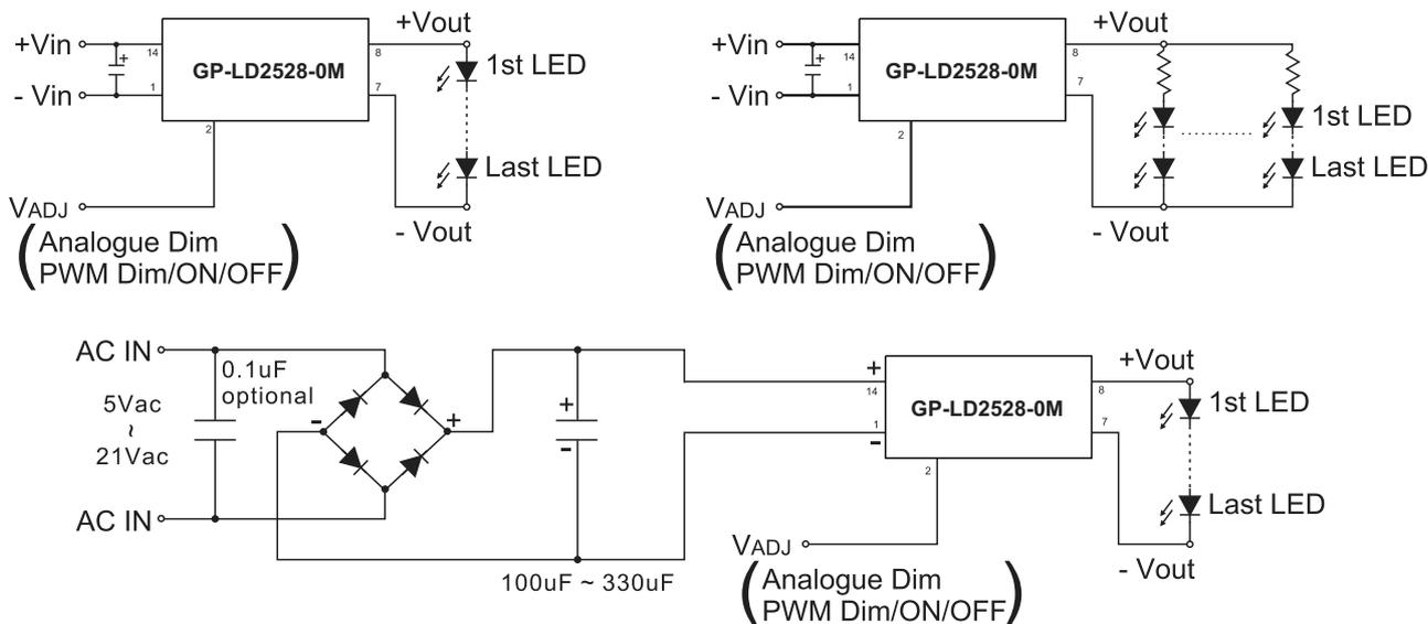
**Output Current Adjustment By External DC Control Voltage**
