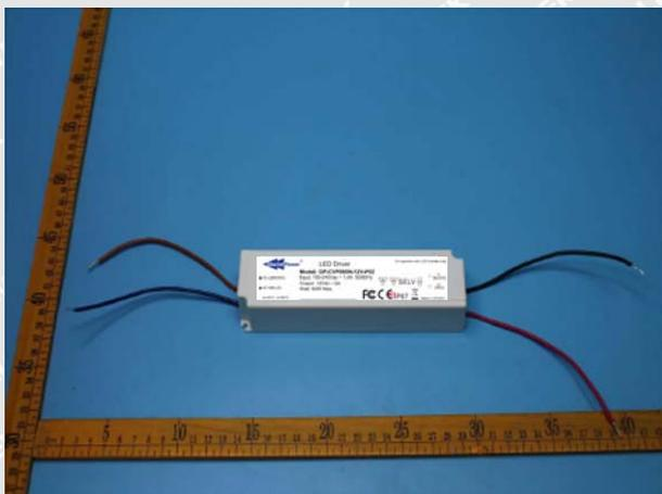
Photo 2 -- During the test of IP6X
