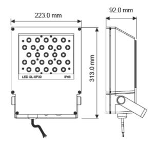
The unique **SP30 Series LED Spotlights,** proudly introduced by **GlacialTech** to the lighting market, use **30W** high power LEDs as the light source and have excellent features, like long lifetime (>30,000hrs min.), high luminous efficacy, and low environmental pollution. They are designed to use an AC source of 100-240V and provide an ideal choice for spotlight/outdoor lighting.
