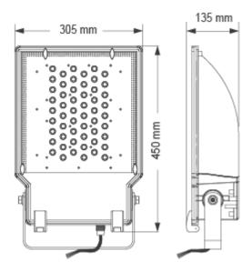
The unique **SD60 Series LED Spotlights,** proudly introduced by **GlacialTech** to the lighting market, use **60W** high power LEDs as the light source and have excellent features, like long lifetime (>30,000 hrs min.), high luminous efficacy, and low environmental pollution. They are designed to use a DC source of 11-15V/22-30V and provide an ideal choice for spotlight/outdoor lighting.
