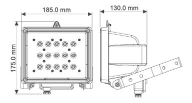
The unique **SD15 Series LED Spotlights,** proudly introduced by **GlacialTech** to the lighting market, use **17W** high power LEDs as the light source and have excellent features, like long lifetime (>30,000 hrs min.), high luminous efficacy, and low environmental pollution. They are designed to use a DC source of 11-15V/22-30V and provide an ideal choice for spotlight/outdoor lighting.
