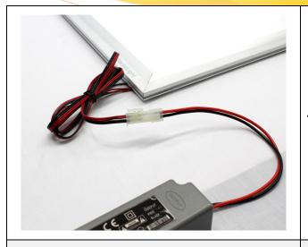
4. The DC power cord connector should be properly connected, not loose.
