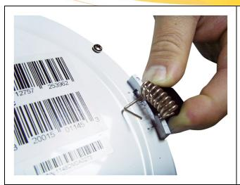
(4.) Squeeze the spring tight and place the other end into the spring holder.
