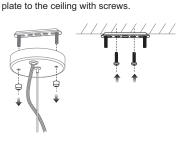
Remove the cap nuts and attach the mounting
