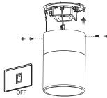
turn off the power before installing.
