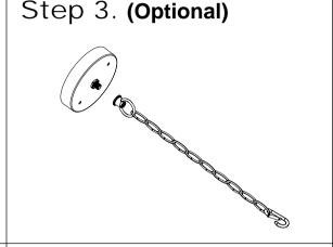
Lock one end of the safety chain to the ceiling mount.
