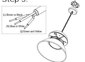
Connect the fixture's power cables to their corresponding colors of the power source and entwine together. Connect the grounding line to the grounding screw of the grounding devices or mounting plate(optional).
