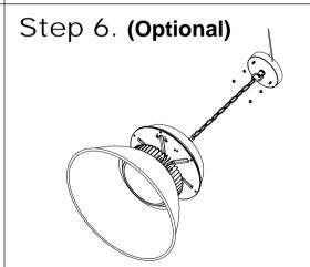
Secure the ceiling mount's cover by screwing the 3/16 nut tight, followed by screwing the 3/16 semi-circular nut tight.
