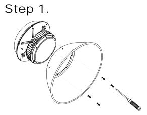
Use four M5\*8mm screws to secure the light-shade to the fixture with a Phillips screwdriver.
