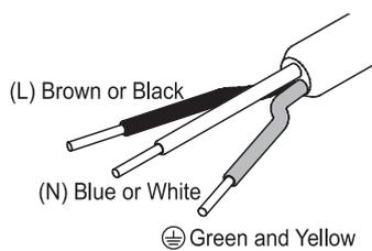
⊖ Grounding line should be fixed perpetually and not allow to disconnect.
