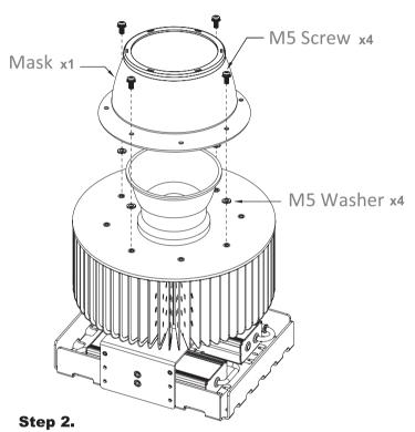
Install the Mask on the lighting fixture using the  $\,$  M5 screws and washers in the order shown Installation complete.
