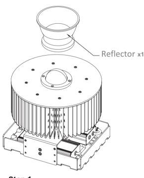
**Step 1.**Center the reflector over the LED.
