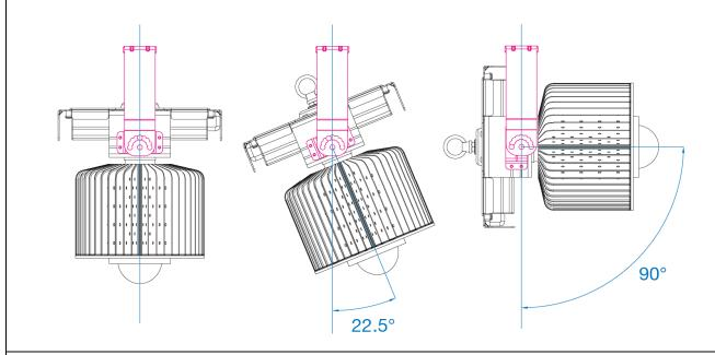
The bracket has a maximum adjustment angle of 180 degrees and can be adjusted into 8 different positions, each one 22.5 degrees apart.
