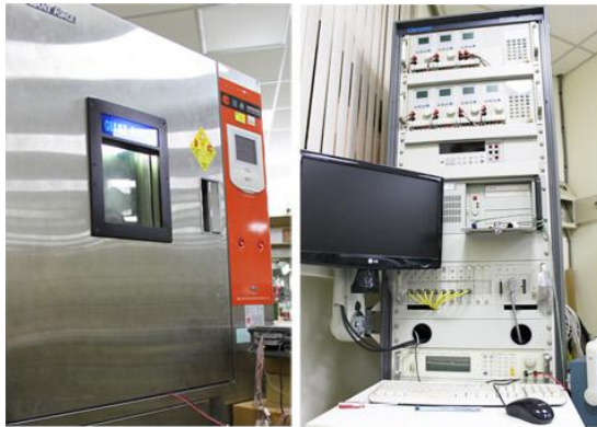
CHROMA model 8000 SMPS auto test system (right) Giant force temperature & humidity chamber (left)
